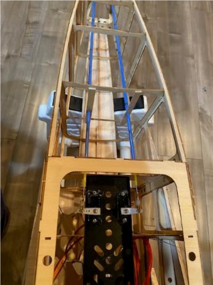
Servo and control linkage set up for the tail feathers.
