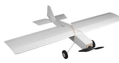
it is made with their white foamboard they call Maker Foam. As a result, you can install lights on the inside of the plane and they will show up quite well. I also installed external LEDs under the leading edge, Red for left wing and Green for right wing. You can find various
