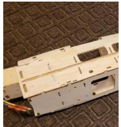
Backing up to that "Paste" picture, I'll share something I learned that led me to believe I wouldn't be turning out a museum piece. This plywood doubler A1-3 is "pasted" to the front portion of each balsa fuselage side. I applied some good ol' Titebond to join the accurately-cut doublers on each side of the fuselage, and after ensuring they were just perfect, I laid some weight on them to make sure everything was good to go.
