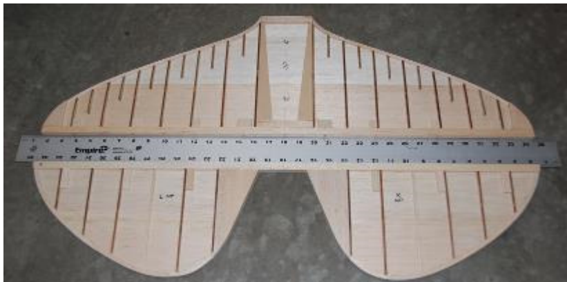
Framed up stab/elevators. Yes, the ruler is 36 inches, not centimeters, long!
