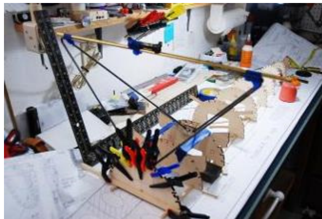
Lower fuselage half with hand bent LG.
